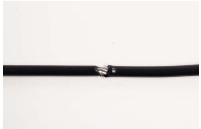
A CRACK IN THE CABLE COVER
