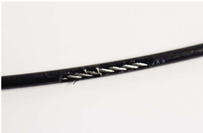
A TEAR IN THE CABLE COVER
