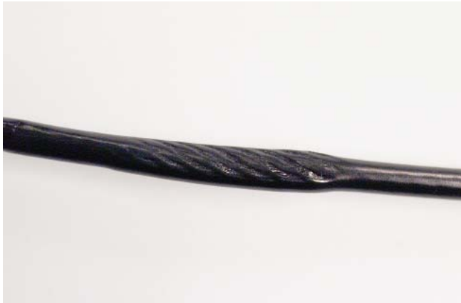
"NECKING", STRETCHED CABLE COVERING
